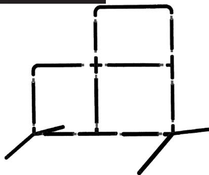
Add net by sliding over top frame. Net should fit like a "pillow case". Use lacing twine provided to secure net opening to bottom rail.
