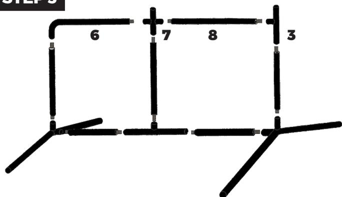
Attach Part #6, Part #7, Part #8 and Part #3 per diagram.
