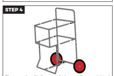
Flip top portion of ball cart upside down on the ground. Attach bottom portion of ball cart to pre-assembled top portion.
