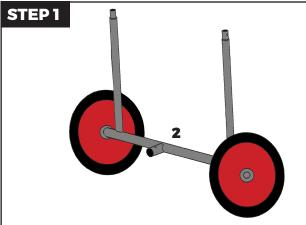
Install (2) Never Flat Wheels to Bottom frame wheel assembly (Part #2). Add Wheel washer to outside of each wheel and secure using Wheel Cotter pins.
