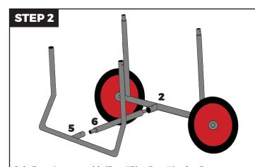
Join Front Leg assembly (Part #5) to Part #2 using Bottom center piece (Part #6) via push button assembly provided.
