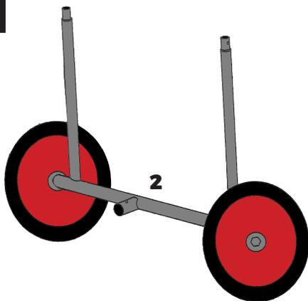
Install (2) Never Flat Wheels to Bottom frame wheel assembly (Part #2). Add Wheel washer to outside of each wheel and secure using Wheel Cotter pins.
