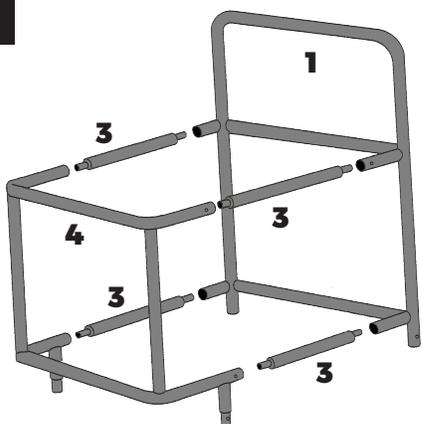
**NOTE: Pre-assemble top portion of ball cart before adding to bottom frame.**
