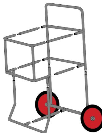
Flip top portion of ball cart upside down on the ground. Attach bottom portion of ball cart to pre-assembled top portion.
