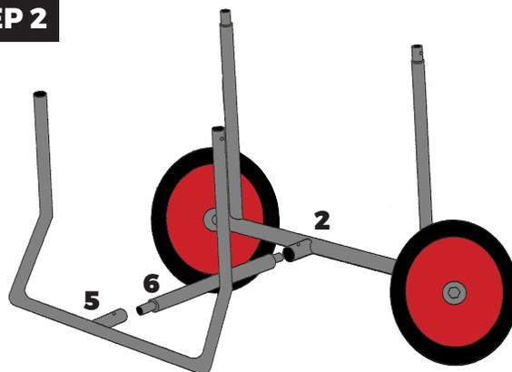
Join Front Leg assembly (Part #5) to Part #2 using Bottom center piece (Part #6) via push button assembly provided.
