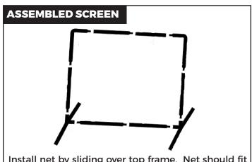
Install net by sliding over top frame. Net should fit like a "pillowcase". Use lacing twine provided to secure net opening to bottom rail.
