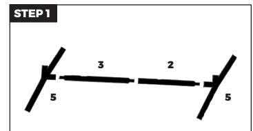
Using diagram shown, start by joining Part #3 and Part #2 with Part #5 4-way leg pieces on each end using push button assembly.
