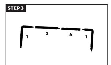
Assemble top half of frame by joining Part #2 and Part #4 with (1) Part #1 elbow pieces on each end.
