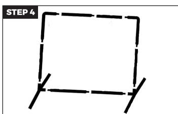
Join top half with bottom half of frame assembly.
