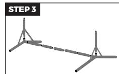
Attach (2) flat support bars to each side as shown. Use 2.5" bolt and nuts to attach to top hole in #2 piece. Use 2" bolts and nuts to attach to bottom portion of legs.
