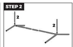
Install (2) #2 male/ male pieces according to diagram shown. Use 2" bolts and nuts to attach to bottom angle bar legs.
