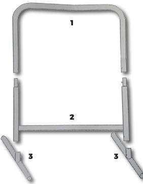
Remove contents from box and use preassembled push-buttons on each side, attach upper frame (Part #1) to lower frame (Part #2).
